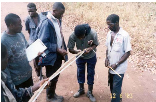
Measuring meter marks on a bamboo for heights; a degraded sawtimber stand.
